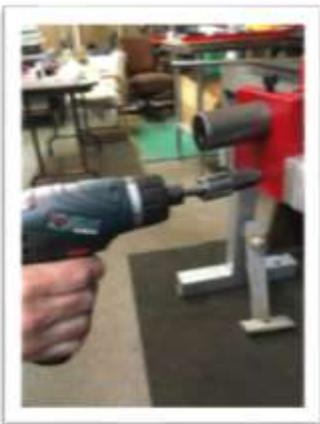
For concave cutting, the rig is to be parallel to the lathe bed. Presumably the hollowing bar from the Clark Deep Hollowing System is switched out with the 12" long holder. Now either the lower or upper setscrews are loosened to allow pivoting. A tool rest must be used to support the bar. Large diameter concave hollowing projects are possible such as platters or large bowls.
