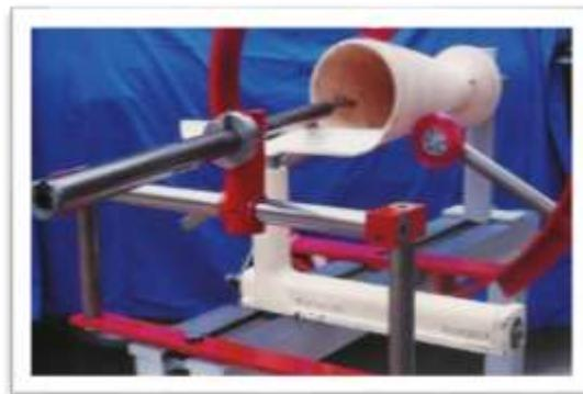
Additional accessories include a handle, adapters to step down the hole in the bar. You can use most must tool bits on the market such as those from John Jordan or the Stewart style (as shown). The base can be mounted close or far away from the wood according to preference.
