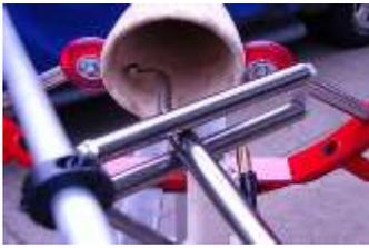
The hollowing bar should be level by adjusting the height of the horizontal cross-bar and the guarded tool rest or other tool rest in the banjo. The base can be slid and angled as desired to approach the hollowing at a wide range of angles not possible with D-handle design. The guarded tool rest is a safety device to prevent the hollowing bar from falling to the ground.
