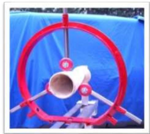
Number two reason for uniqueness relates to the ring design which limits loss of the maximum swing diameter possible on a lathe. Other common designs use a vertical ring, which subtracts at least 4 inches from maximum swing diameter at the point supported by the steady rest. The only loss to maximum diameter in this steady comes from the ½ inch base plate. Even the attachment bolt is recessed in the base plate to keep it from interfering with turning diameter.
