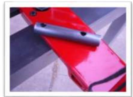
aligned to pass through the holes. Slide the hollowing bar through the horizontal bars of the guarded tool post. Slide the larger split rings onto the hollowing bar placing one at the far rear of the bar and one in front of the swivel device (on the side of the headstock) at the mid-point of the bar (24 inches from the end). Insert the aluminum laser holder into the smaller split rings.
