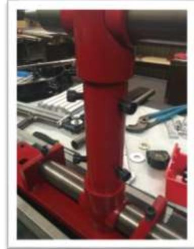
Position the distance of the cutter by turning the leadscrew with a 5/8" socket
