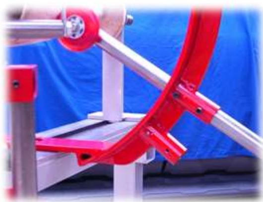
On the left is an photograph of a ‘Multi-Steady’ that has two pairs of through tubes with one set aimed at 10 inches and the other at 12 inches over the base plate. It can be used on two different sized lathes such as a 20” Powermatic and a 24”Oneway. A third set of tubes can also be added so the Clark Multi-Steady could be used on a 16, 20 or 24 inch swing lathe.
