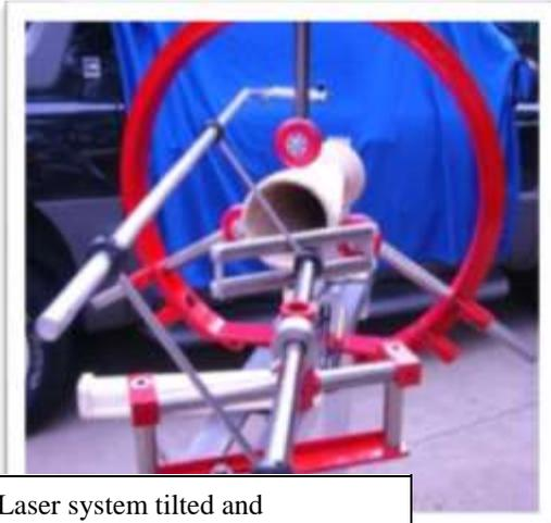
Laser system tilted and articulated to pass around steady rest radial arm at 12 o'clock
